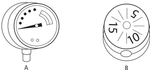
Figure 6. (A) Dial gauge. (B) Weighted gauge.
